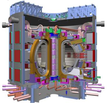
Plasma is confined by toroidal magnetic field.
