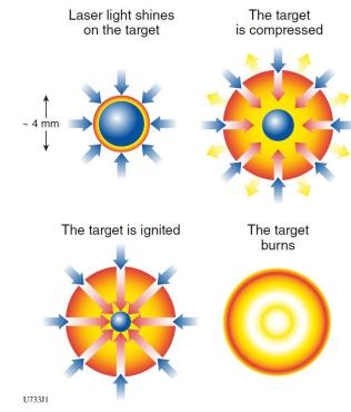
A DT ice capsule filled with DT gas is imploded by laser.
