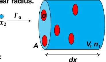
Fraction of total area blocked by targets is:
