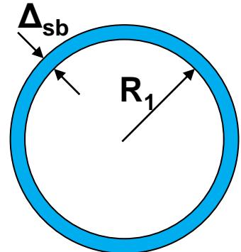
$$IFAR = \frac{R_1}{\Delta_{sb}} = \frac{R_1}{\frac{M}{\rho_{sb} R_1^2}} = \frac{\rho_{sb} R_1^3}{M} = \frac{\rho_{sb}}{M} \frac{Mu_{max}^2}{p}$$
