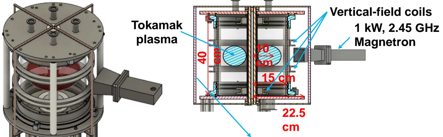
4 toroidal-field coil connected in series. Two turns in each coil. 2.5 kA pulsed-current.  $B=876$  G @ 4.6 cm will be used for ECR heating.
