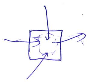
A fluid element at a fixed spot in the cup, retains its identity although particles continually go in and out of it.
