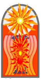
Compressed and heated, lithium-6 deuteride fuel begins fusion reaction, neutron flux causes tamper to fission. A fireball is starting to form...
