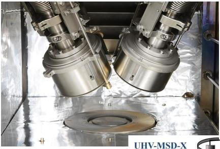
Rotatable Manipulator Sample Stage Substrate Thickness Monitor Thin Layer **Gas Shower** Head . Gauge Cathode Shielding Magnetron DC/RF Power Magnetron Cathode
