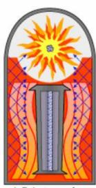
Polystyrene foam becomes plasma, compressing secondary, and plutonium sparkplug begins to fission.
