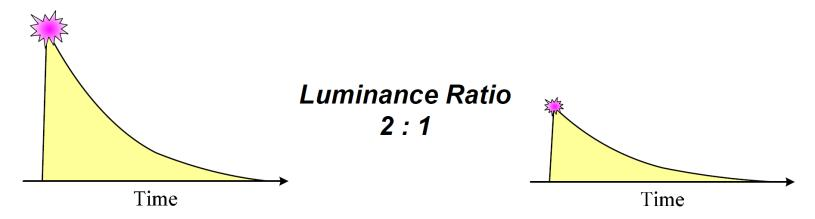
PDP : Control the Luminance using Number of Light Pulses
