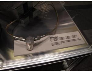
**Project Y Atomic Bomb Detonator System Spark Gap Switch**
