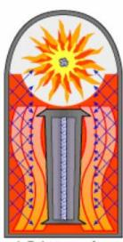
Polystyrene foam becomes plasma, compressing secondary, and plutonium sparkplug begins to fission.
