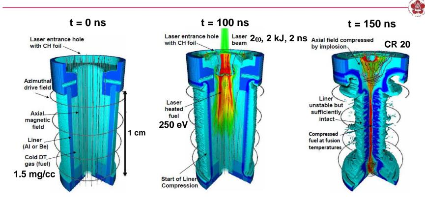
The stagnation plasma reached fusion-relevant temperatures with a 70 km/s implosion velocity
