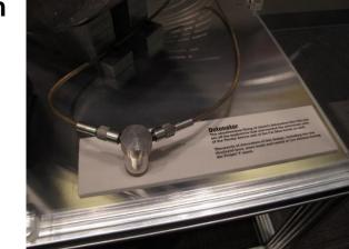
Project Y Atomic Bomb Detonator System Spark Gap Switch
