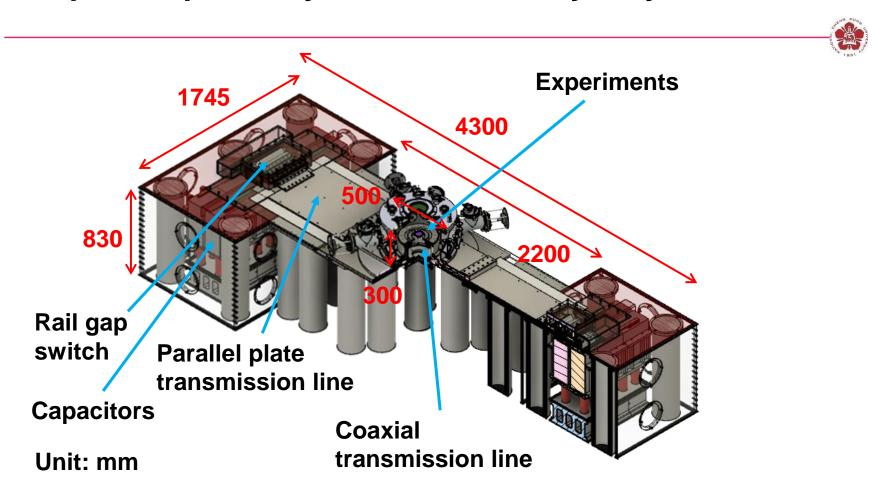
A 1 kJ pulsed-power system at ISAPS, NCKU started being operated since September, 2019.
