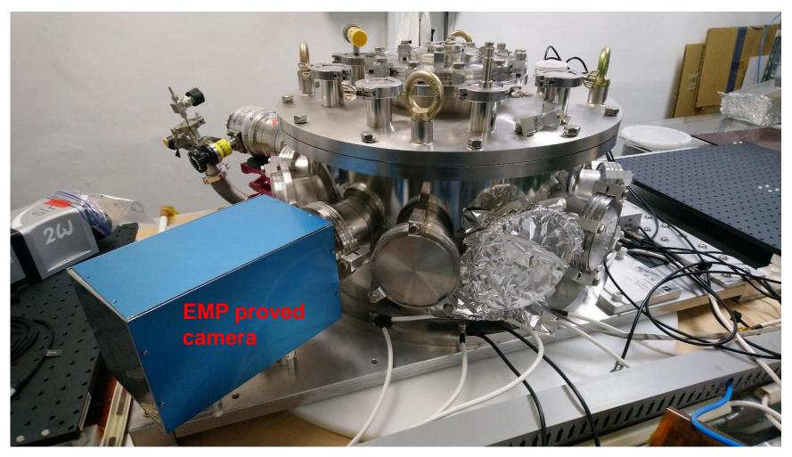
• The camera is controlled via wifi and powered by batteries.
