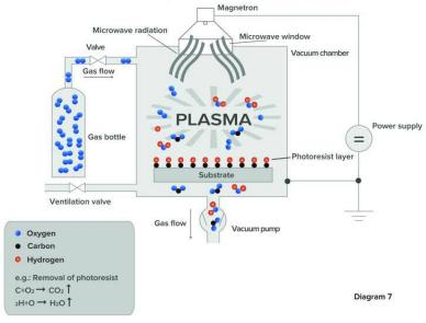
Low-pressure plasma system: Cleaning with a microwave generator
