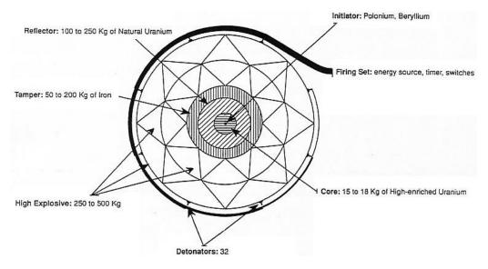
Small-scale slow-motion cross-section of a shaped charge implosion design
