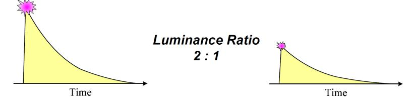
• PDP : Control the Luminance using Number of Light Pulses
