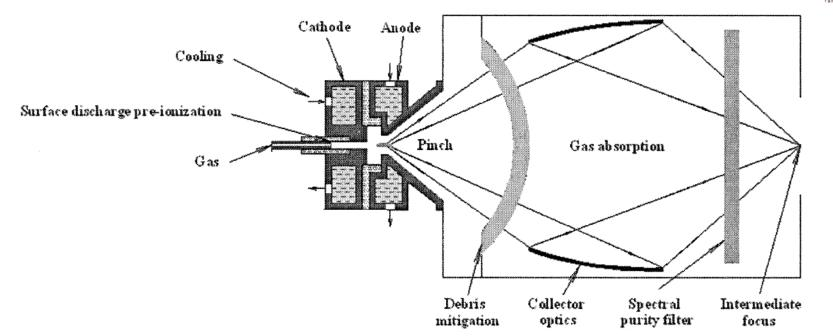
• Electrodes are damaged significantly due to the heat and sputtering by ions.
