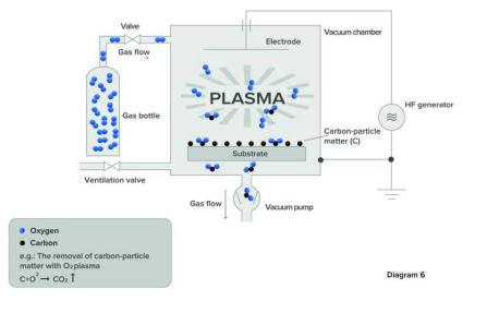
Low-pressure plasma system: Generation with a low-frequency or high-frequency generator
