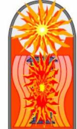
5. Compressed and heated, lithium-6 deuteride fuel begins fusion reaction, neutron flux causes tamper to fission. A fireball is starting to form ...
