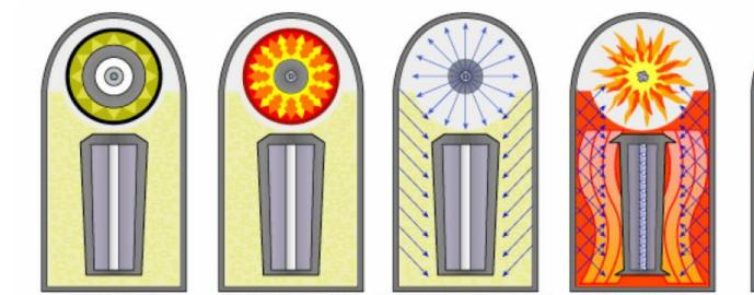
1. Warhead before firing; primary (fission bomb) at top, secondary (fusion fuel) at bottom, all suspended and beginning a fission in polystyrene foam.
