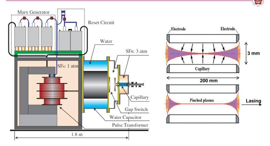
If 200~500 mTorr Ar is used as the filled gas, 46.9 nm (26.5 eV) Ne-like Ar laser can be built.
