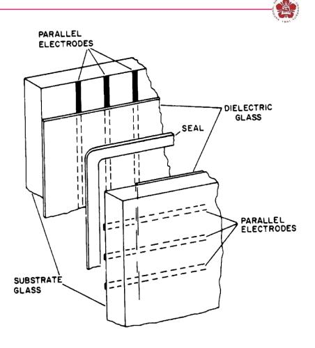
It could be baked under vacuum at 350 °C to drive out contaminants.
