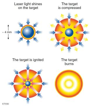
A DT ice capsule filled with DT gas is imploded by laser.
