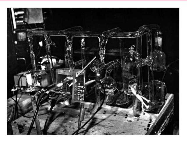
• It had the same alternating sustain voltage, neon, gas, and dielectric glass insulated electrodes that are used for plasma TVs today.
