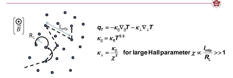
Typical hot spot conditions: R<sub>hs</sub> ~ 40 μm, ρ ~ 20 g/cm<sup>3</sup>, T ~ 5 keV: B > 10 MG is needed for χ > 1
