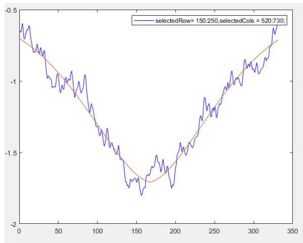
Figure 126: X軸:pixel Y軸:phase. Plasma plume, 40ms delay, average of cols 520~750, average of row 150~250
