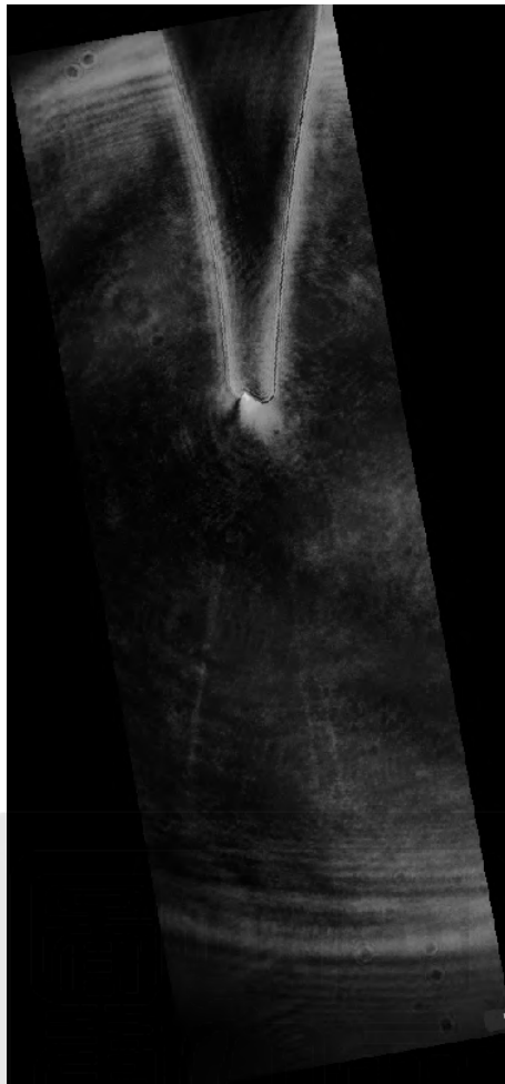
Figure 37: Schlieren image captured in vacuum environment with gas jet - cutline 600.
