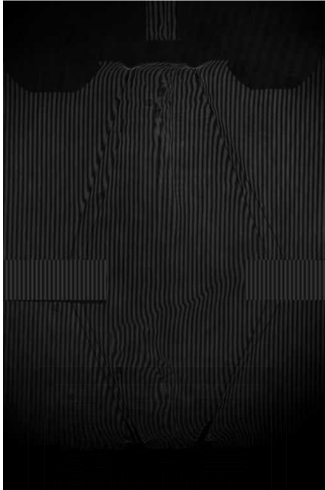
Figure 35: The middle wire support cover by the generated interference fringes 03/30.
