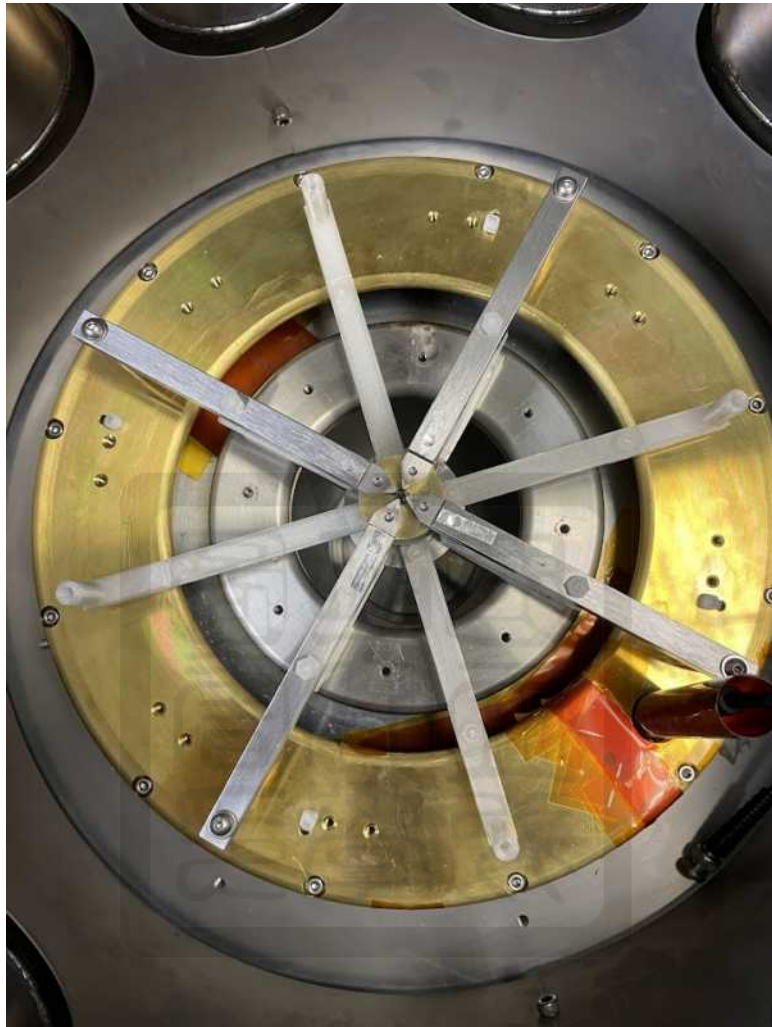
Figure 12: top horizontal support 固定於 top support 上，輔助支架未拆
