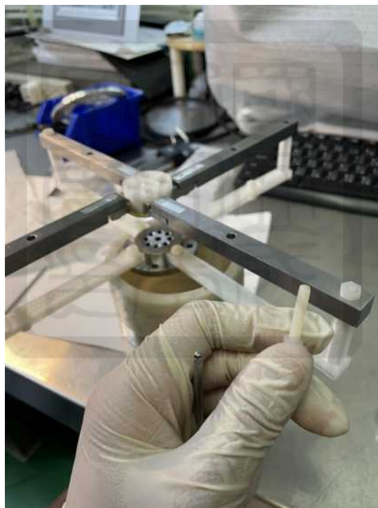
Figure 7: top horizontal support固定於輔助安裝支架
