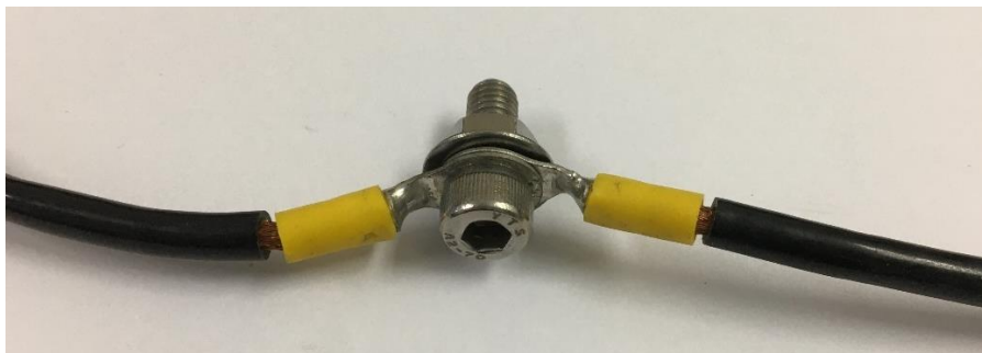
Figure 4.3: The connection of toroidal magnetic field coils.
