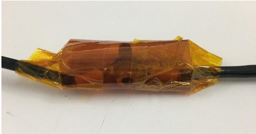
Figure 4.4: The Kapton and Kapton Tape to wrap up the parts of metal.
