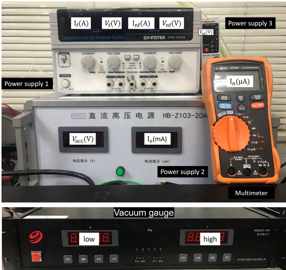
Figure 27: Power supply system of MIT-MEB.
