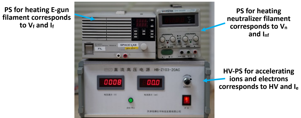
Figure 5.4: Power supply system of MIT-MEB.
