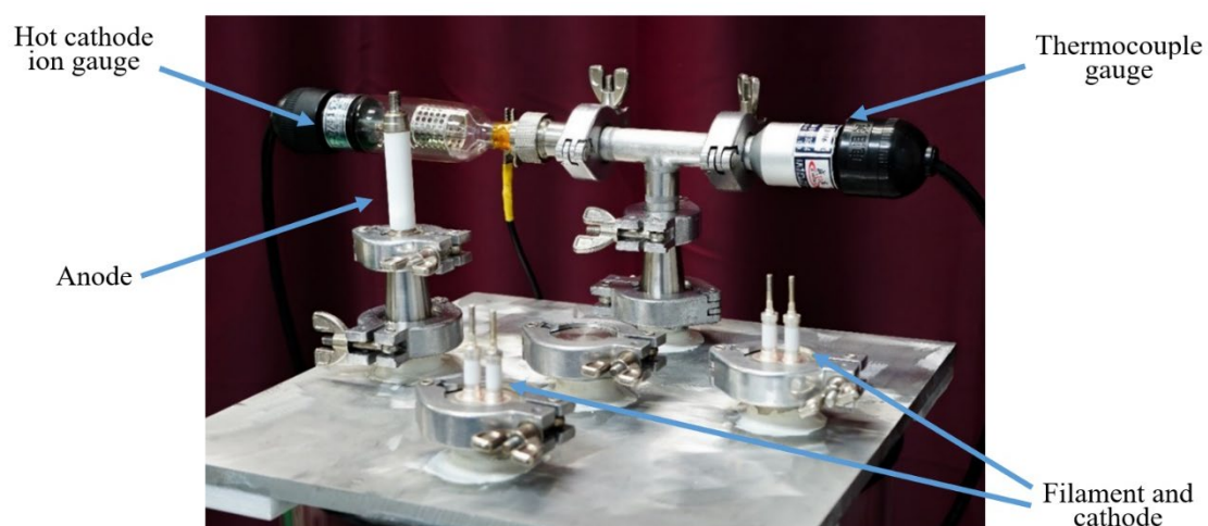
Figure 4.10: Configuration of top cover plate.
