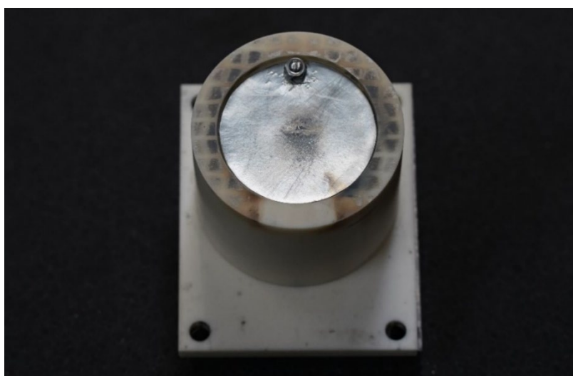
Figure 7.2: Zinc vapor projection on the evaporator.
