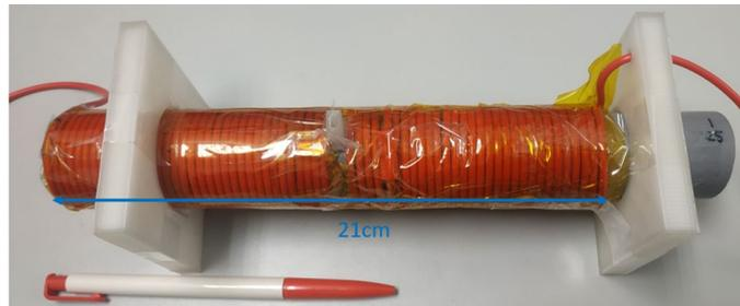
Figure 30 The picture of the solenoid.
