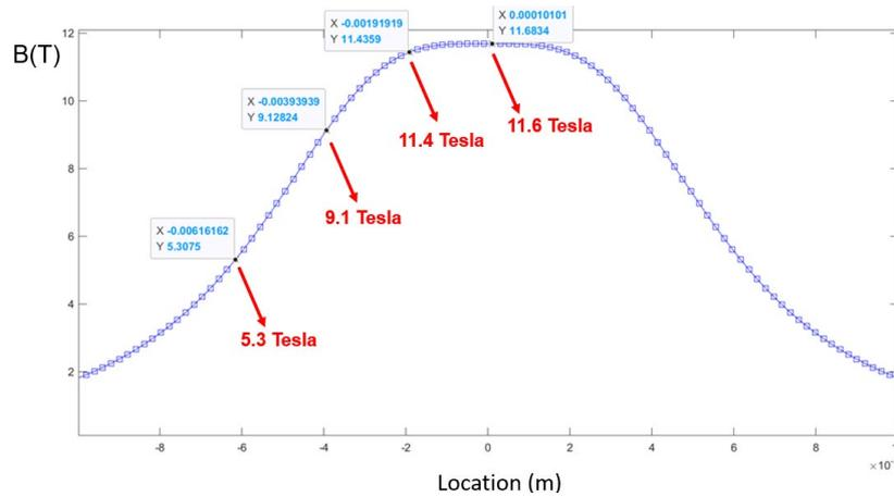
Figure 5 The axial magnetic field distribution of this Helmholtz coil.
