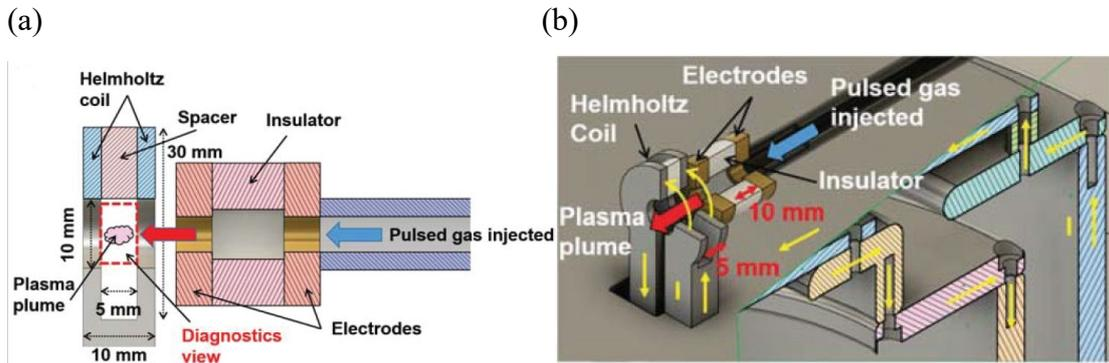
Figure 1 (a) The side view of the Helmholtz coil for the theta pinch. The gap between two coils provide a clear view for diagnostics. (b) The schematic of our proposed EUV light source.
