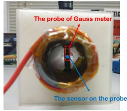
Figure 33 The probe of the Gauss meter is fixed in the center of the circular section of the solenoid.
