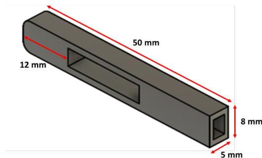
Figure 32 The CAD drawing of the support.
