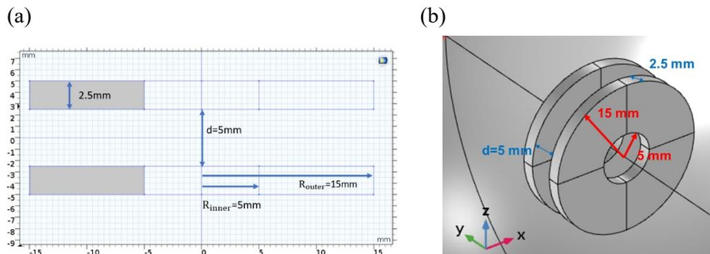
Figure 12 (a) The planar structure of the Helmholtz coil. (b)The three-dimensional structure of the Helmholtz coil.
