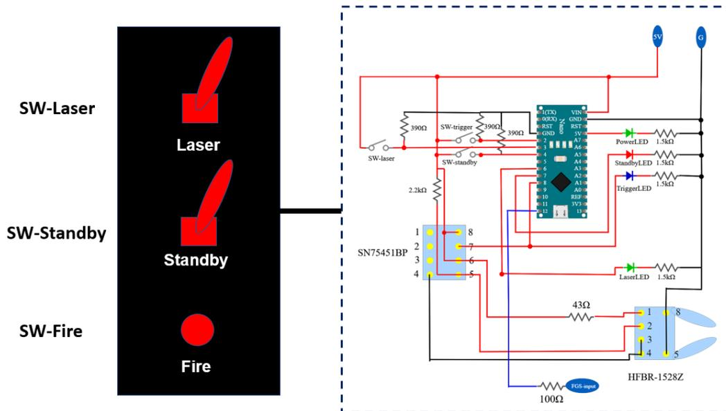
Figure 44 The circuit of the new optical trigger-pulse generator.
