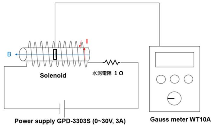
Figure 34 The circuit of the experimental set up.
