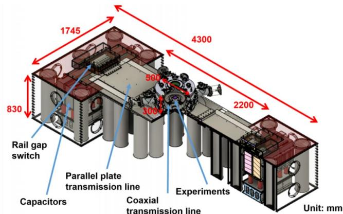
Figure 15 The CAD drawing of the Our pulsed-power system [3].
