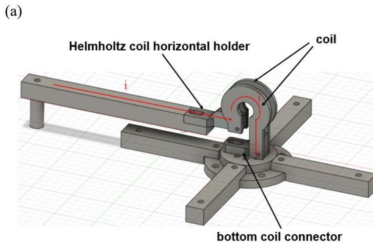
Figure 3 (a) The CAD drawing of Helmholtz coil.
