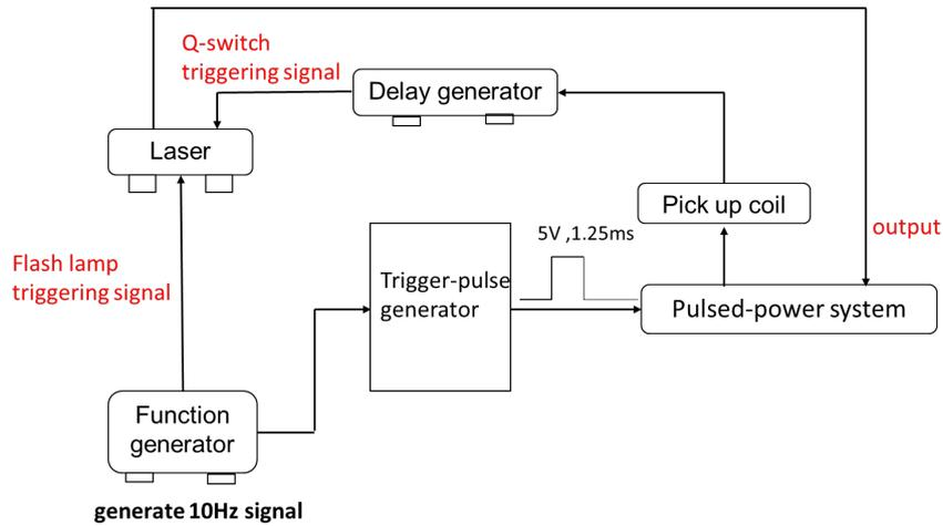
Figure 41 The relation chart of triggering the system
