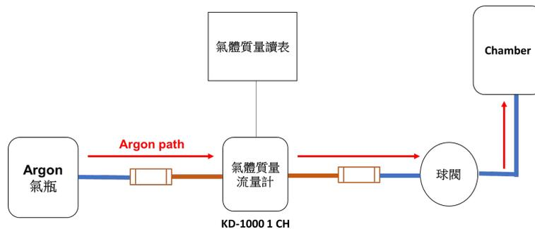
Figure 21 The path of argon gas flow in the system.
