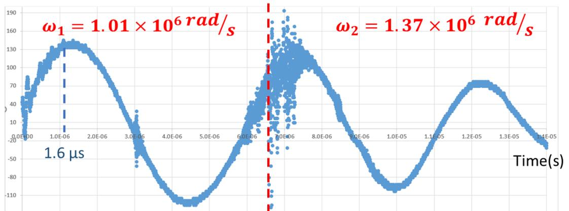
Figure 27 The one of the discharge currents measured with the Rogowski coil.
