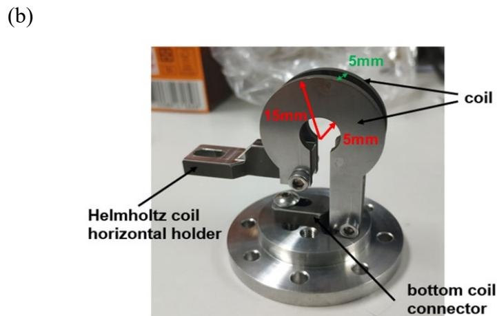
Figure 3 (b) The picture of Helmholtz coil.
