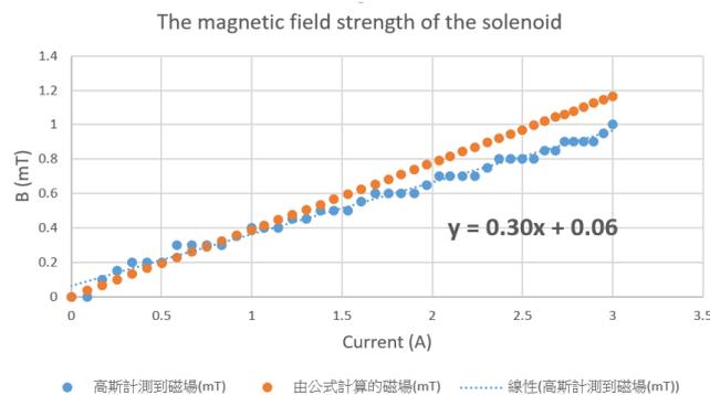
Figure 35 The results of the magnetic field generated inside the solenoid.
