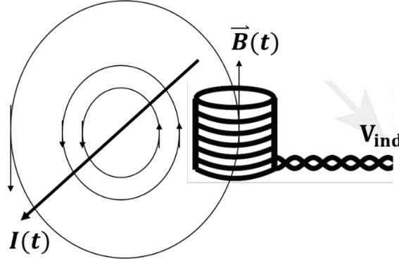
Figure 28 The schematic of the B-dot probe [6].
