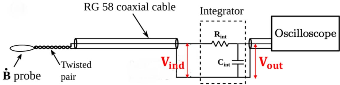
Figure 29 The circuit of the B-dot probe with a integrator.
