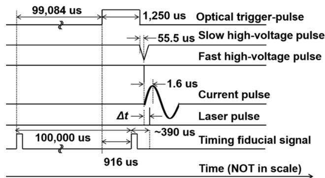
Figure 42 The time sequence of triggering the system [9].
