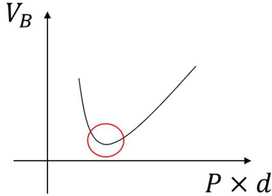
Figure 22 The schematic of the Paschen 's curve.
