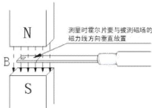
Figure 31 The way to measure the magnetic field with the Gauss meter [8].
