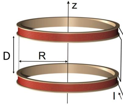
Figure 2 The Schematic of one-axis Helmholtz coil [1].
