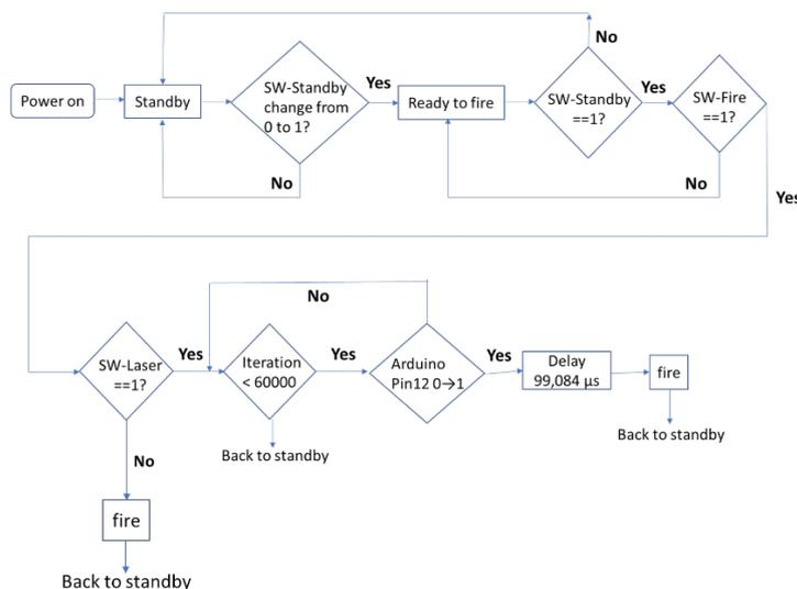
Figure 45 The flow chart of the new optical trigger-pulse generator.
