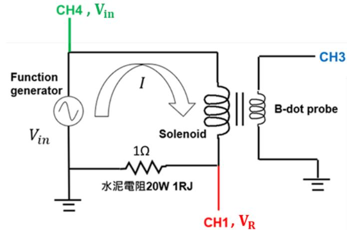
Figure 37 The circuit for calibration of the experiment.
