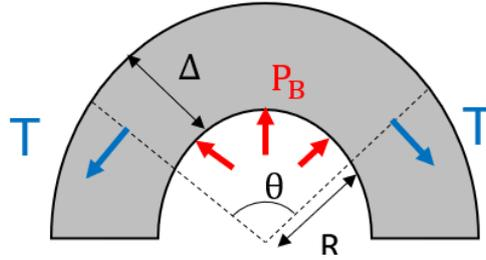
Figure 4 The relation between the tension on the coil  $T$  and the magnetic pressure  $P_B$ .
