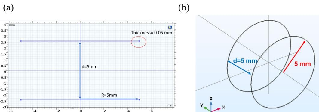
Figure 10 (a) The planar structure of the Helmholtz coil with small thickness. (b) The three-dimensional structure of the Helmholtz coil with small thickness.
