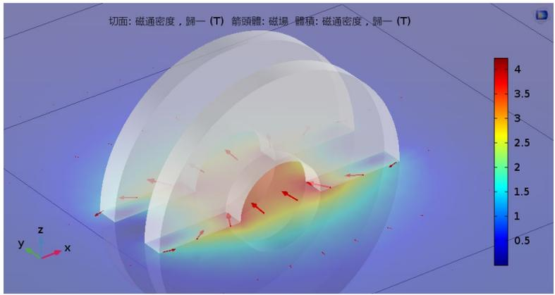
Figure 13 The magnetic field distribution of the Helmholtz coil.
