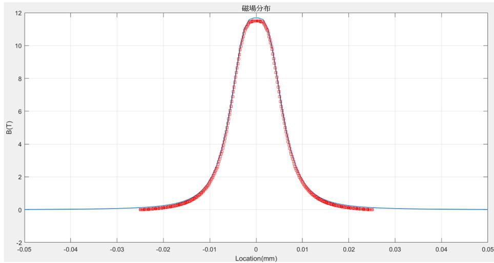
Figure 11 The comparison between the axial magnetic field of the simulation and the theoretical calculated axial magnetic field.
