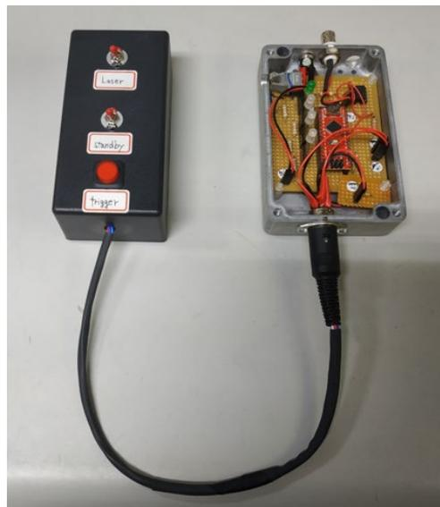
Figure 43 The photo of the new optical trigger-pulse generator.
